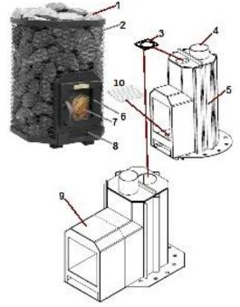
Figure 1. Heater components
